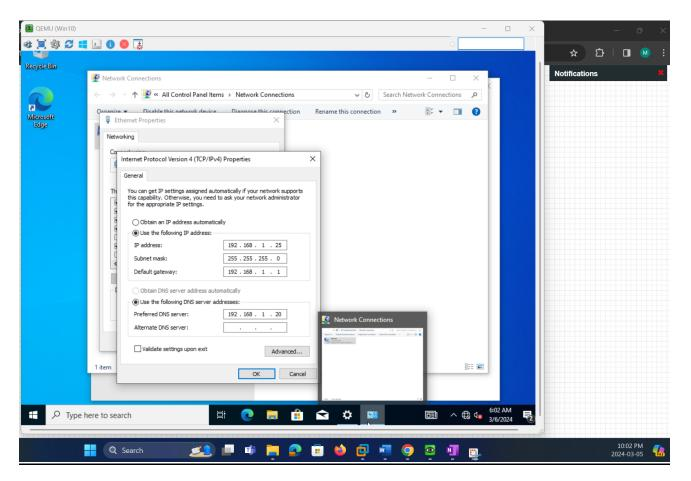
The network configuration settings of the Windows 10 client, where a static IP address has been assigned to the machine to ensure consistent network communication within your domain environment. It's also set to use the Windows Server 2016 machine as its preferred DNS server, indicating integration with the domain for DNS resolution.
